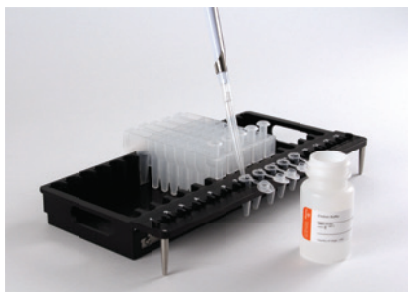
Figure 2. Setup and configuration of the deck tray(s). Elution Buffer is added to the Elution Tubes as shown. Plungers are in well #8 of the cartridge.
